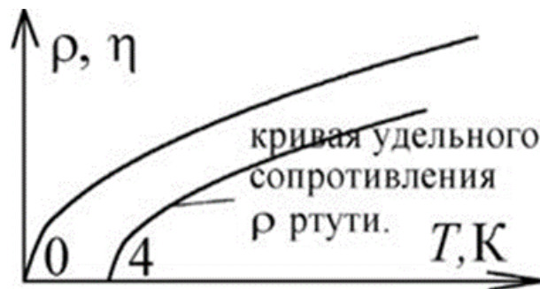
Fig. 177. The viscosity of the gas with decreasing temperature T drops to zero, just like the resistance of the metal, proportional to the viscosity of the electron gas.
