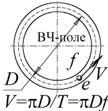
Fig. 48. Direct calculation of the speed V of an electron in a synchrotron gives V > c .
