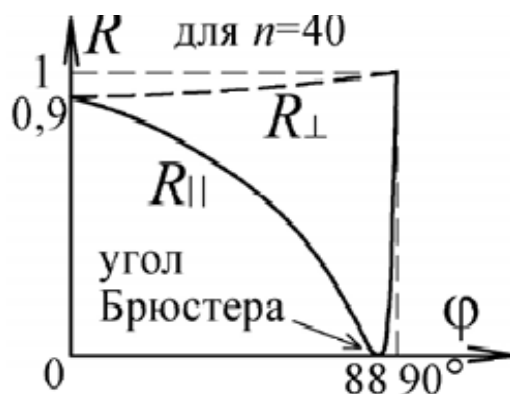
Fig. 154. Dependence of the reflection coefficient R on the angle of incidence \varphi for two types of polarization [74].
