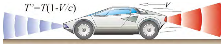
Fig. 26. Doppler effect - a change in the frequency of light due to movement.
