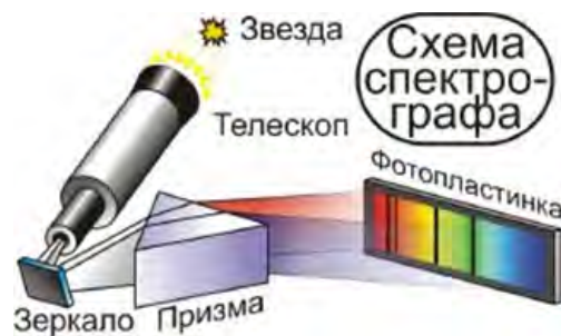
Fig. 55. Study of the spectra of stars using a spectrograph that decomposes light into a rainbow strip with dark absorption lines. The velocity of objects is found from the displacement of the spectral lines.
