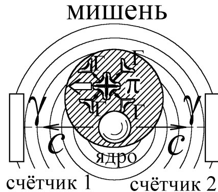
Fig. 136. Bombardment of a hydrogen target, emission of pions, their decay into gammon and emission of gamma rays.
