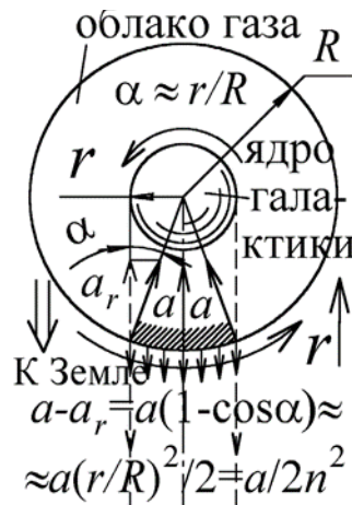
Fig. 60. Re-emission of the light of the nuclei by a rotating cloud of gas gives a shift of the lines without their broadening.
