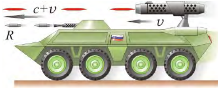
Fig. 20. Ballistic principle: an increase in the speed of a light beam by the value of the speed v of the source. An analogy of firing a machine gun and a ray gun from an armored car on the move.
